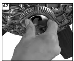
Install center plug by turning in direction of arrow till tight.
